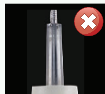
Worn screw thread with non genuine tips
